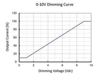
This system connects to your LED fixture, which allows you to choose the right light level based on your need of the moment. For example, at OV, the light will dim to its minimum level, but you will typically need a light switch to turn off the light completely.
